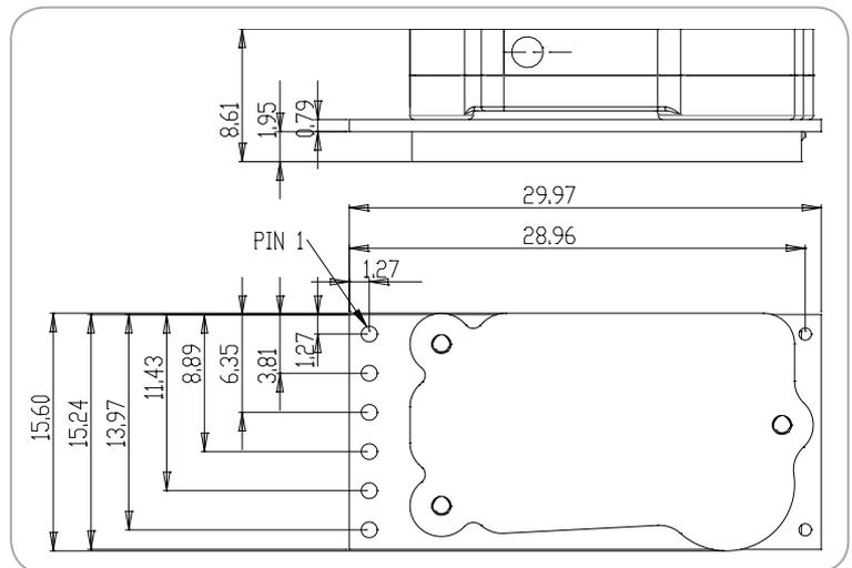
All dimensions in millimeters (mm)
